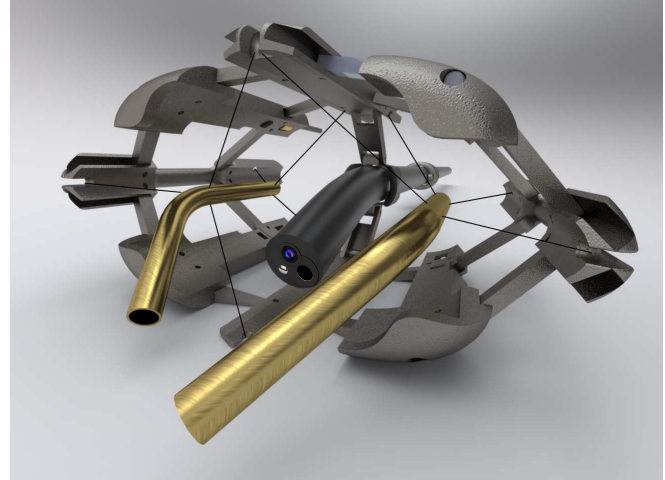
Fig. 1. Render of the ESD CYCLOPS system, without the soft silicone sleeve.
