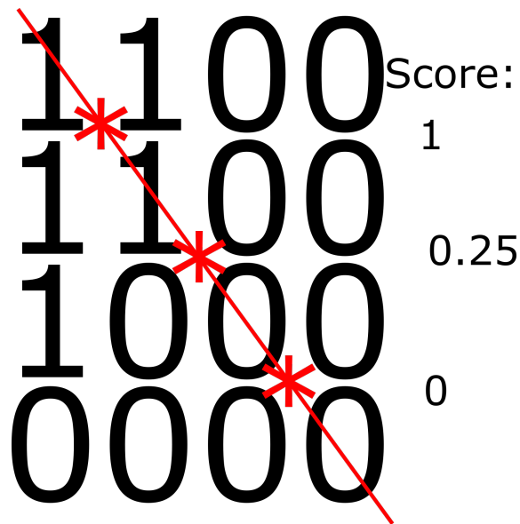
Figure 6.2: Ray intersection with segments, represented as binary (0 and 1) arrays, were checked as follows. Rays are represented as a set of 'ray-points' (red stars) that form a line. Scores at each ray-point were linearly interpolated from the values of the surrounding voxels. Each ray-point's score is multiplied by the interval between ray-points, and summed to generate a path length of intersection for the entire ray.
