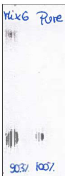
Supplementary figure 21: ITLC-SG strips of ^{89}\text{Zr-DFO-PD-L1}_{\text{mAb}} used for the study presented in Fig.6-6 and 6-7. The ITLC-SG image shows samples of ^{89}\text{Zr-DFO-PD-L1}_{\text{mAb}} pre- (left) and post-purification (right), while dots at the bottom of the strip indicate ^{89}\text{Zr-DFO-PD-L1}_{\text{mAb}} product (loading site) and the black smear at the upper end of strip indicates free ^{89}\text{Zr} (solvent front).
