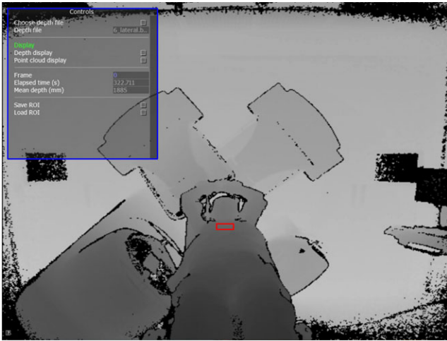
FIG. 3. Screenshot of custom C++ software used to record Kinect depth data. Software controls for manipulating depth frame data are shown in the top left (blue rectangle). A patient is visible on the couch, supported by a breast board. The entire depth frame from the sensor is recorded at a resolution of 512 \times 424 pixels and frame rate of 30 fps into a lossless binary file for later analysis. The user selects a ROI (red rectangle) on the patient's upper sternum region, with an area of approximately 300 pixels. The mean distance from the Kinect v2 to this ROI is then calculated as a function of time to form a breathing trace signal.
