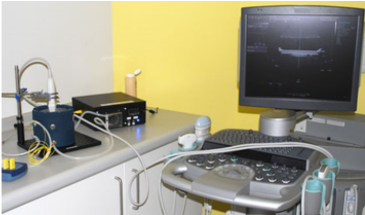
Photograph of maternal-foetal Phantom ISUOG setup. 30x17mm (300 x 300 DPI)
